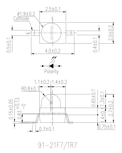
Note: The tolerances unless mentioned are  $\pm 0.1$ , unit=mm.
