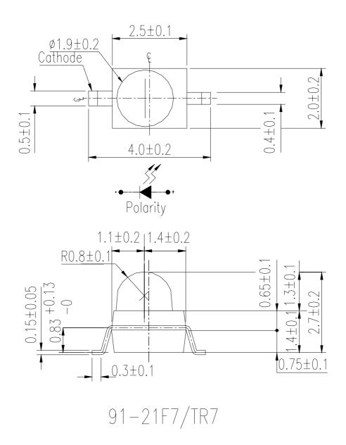
Note: The tolerances unless mentioned are  $\pm 0.1$ , unit=mm.
