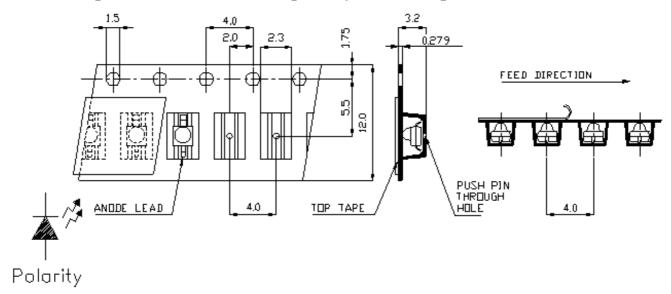
Note: Tolerances Unless Dimension is  $\pm 0.1$ mm, Unit = mm
