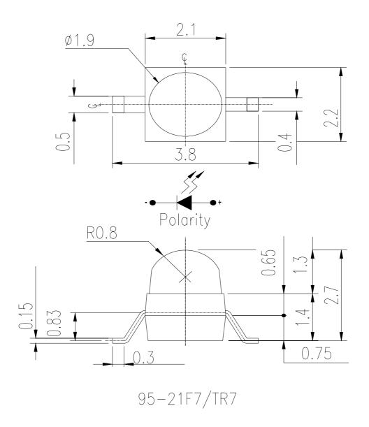
Note: Tolerances Unless Dimension is  $\pm 0.1$ mm, Unit = mm
